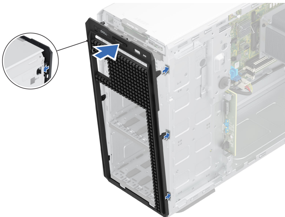
Figure 97. Installing the front faceplate
